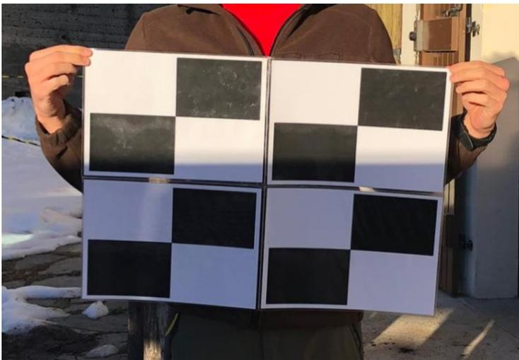
*Figure 5. Chequered sheet used for calculations of CTs' visual clarity index.*
